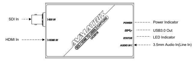
Note: When both SDI and HDMI are plugged, SDI input signal will take priority. When both SDI/ HDMI IN and AUDIO IN are plugged, external audio input will take priority.
